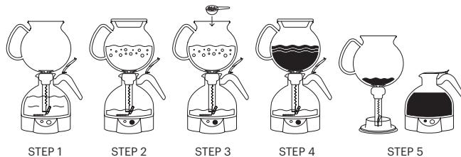
**Note:** If the jug (11) is empty, the appliance will not switch on for safety reasons, in order to prevent the heating element from running whilst dry.
